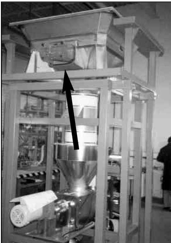
SCR-500 on Box Dumper to prevent hang-ups.
